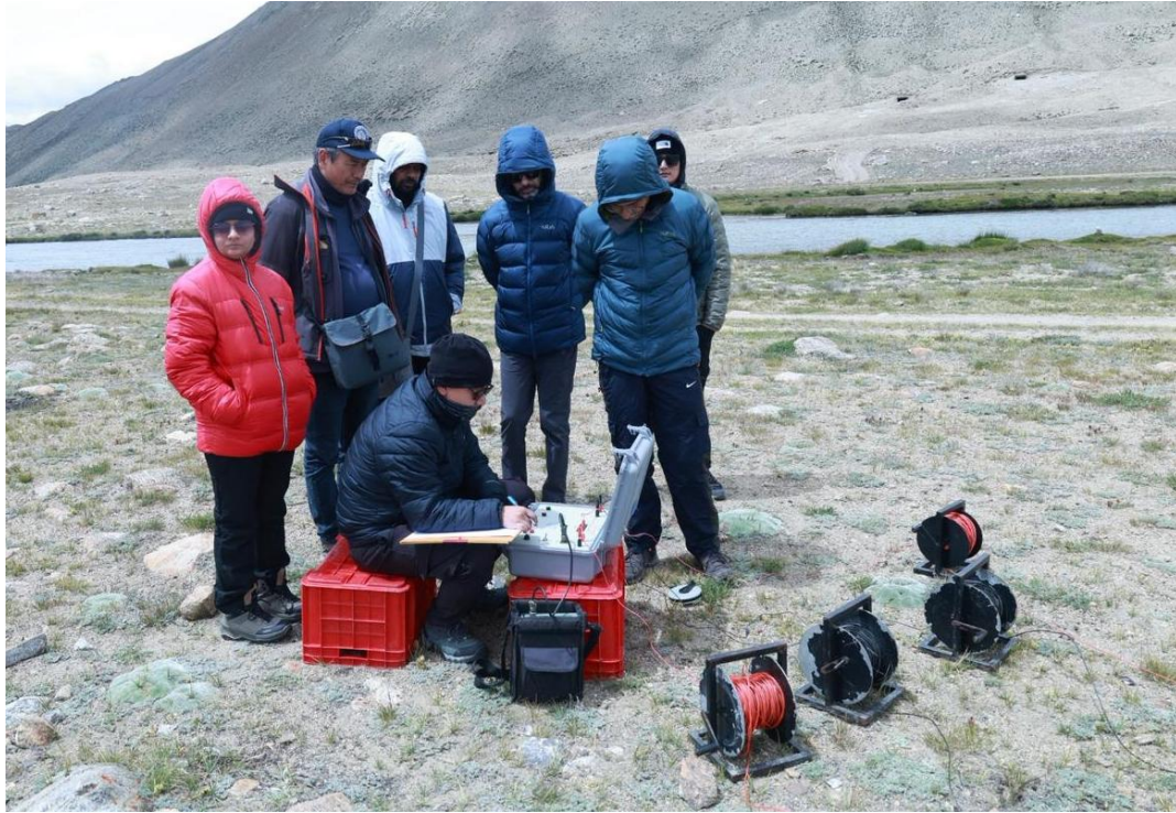
Figure 6: Subsurface geophysical assessment using ERT at Sora Funnel
