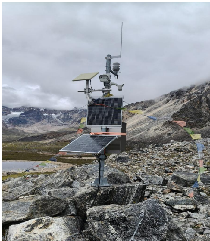
Figure 4: AWS installed at Shako Cho Lake on Right Moraine
