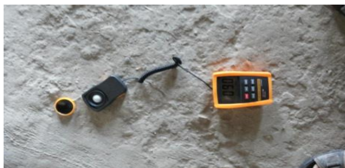
Fig.30 luxmeter indicating 90 lux an insufficient illumination(GSSS Kot)
