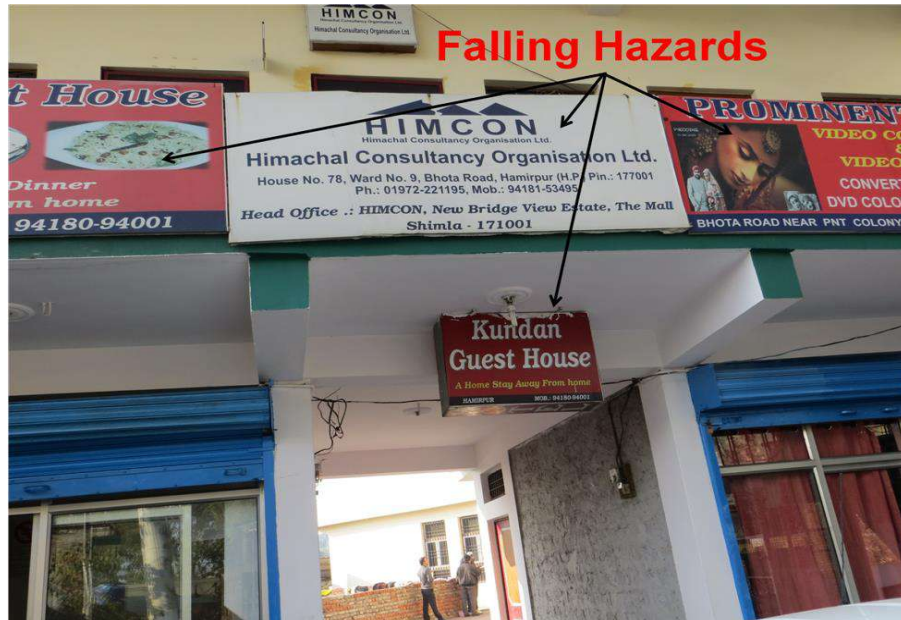
Figure 41: Falling hazards in a building
