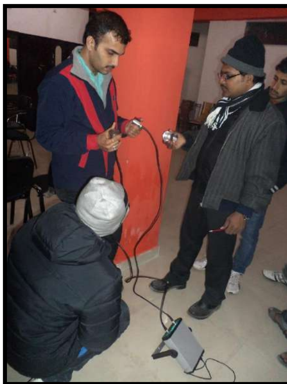
Figure 74: Ultrasonic Pulse Velocity Method (Kangra, 17th December 2013)
